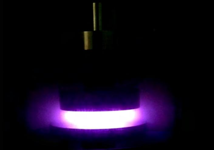
Figure 1: Photograph of the argon plasma used in the project.
